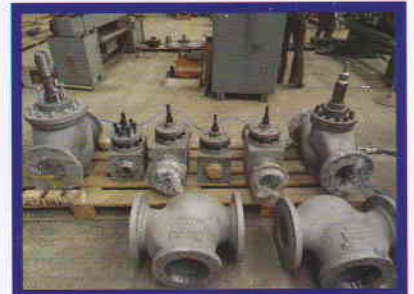
Spray water valves
