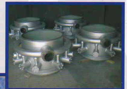
Dump tubes with spray water injection
