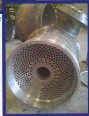
Outlet of Hp Bypass valve
