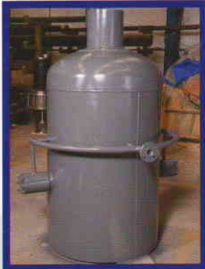
Dump tube with spray water injection
