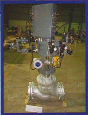
Control valve with junction box and accessories
