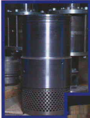
Plug of Bypass valve
