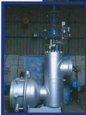
Side view of Bypass valve Z shape in F 91 material
